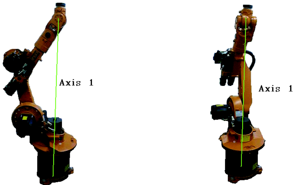
Figure 6: Two KUKA KR-15/2 shoulder singular configurations.
